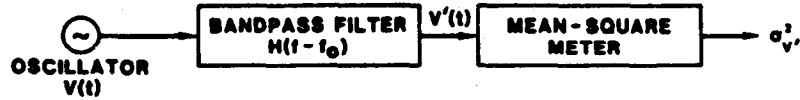
FIG. 12-1 An rf spectrum analyzer. The device produces an output proportional to the mean-square value of the signal passing through a tunable narrow-band filter centered at frequency f_0 .
